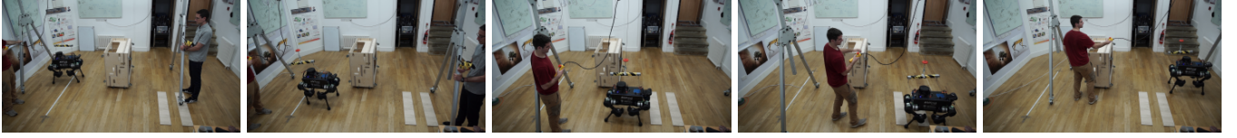
Fig. 5: Utopian trajectory executed on the real robot (same scenario as the simulated “Steps & barrier”). Left to right: footsteps over bump, fast trotting within line of sight, slow walking over the wooden planks, sideways trot to the goal pose.
