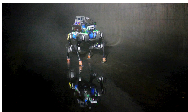
Fig. 1 An ANYmal robot (Hutter et al. (2016)) in a sewer with two feet in a slippery, wet depression and two feet in a dry, elevated area. With prior information about terrain type and geometry, it is possible for the robot to localized in the world using only touch. This would be extremely useful in dark and foggy environment (Image courtesy of RSL/ETH and from Kolvenbach et al. (2020)).
