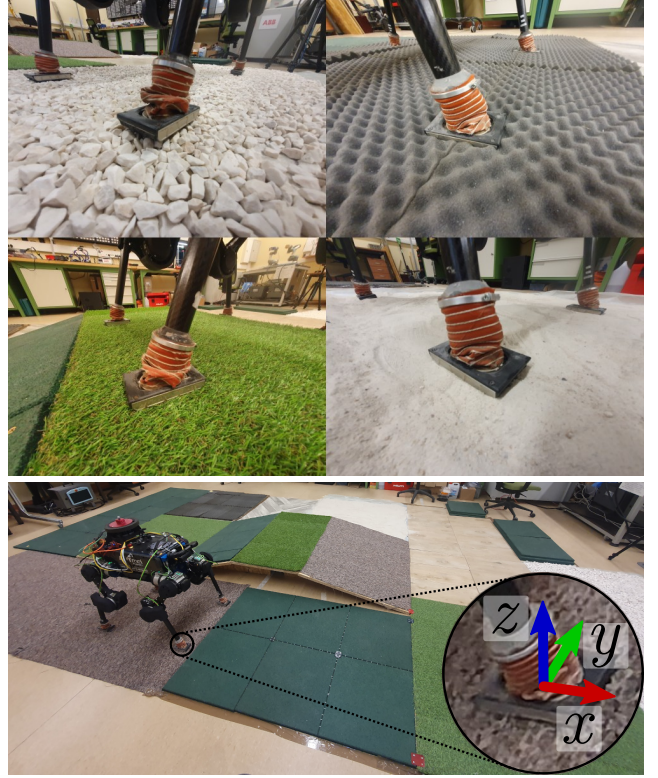
Fig. 10 Top: Examples of foot positioning when collecting data on different terrains under controlled laboratory conditions. Bottom: Experiment 3: ANYmal with sensorized flat feet standing on the multiple terrain type course. Close up of the foot is provided. An IMU and fore/torque sensor is located in the sole with coordinate frame shown.
