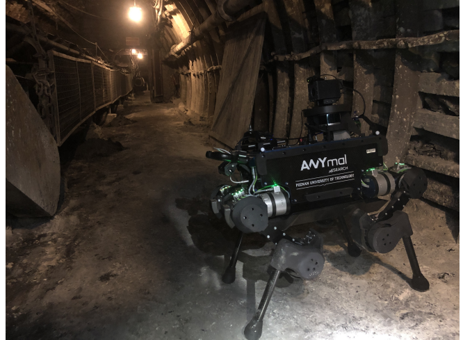
Fig. 1: An ANYmal B300 quadruped robot performing an inspection of conveyors 800 m underground. The failure of vision or LiDAR-based localization can happen due to hot, humid, and dusty working conditions. Our system can increase the robustness of the robot in these repetitive tasks.
