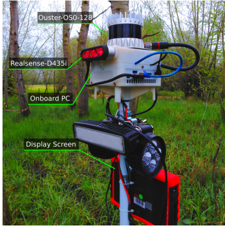
Figure 2: The handheld device used in our system. The labelled components work together to provide online feedback on the forestry data collection
