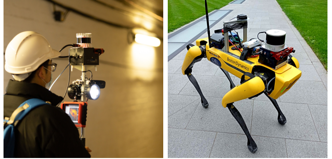
Fig. 1. Two of the platforms used in this work. Left: handheld device including a SevenSense AlphaSense visual-inertial sensor. Right: the same device mounted on a Boston Dynamics Spot quadruped. An IMU bias model from a neural network trained on handheld data was used to infer the biases on the Spot dataset without any retraining — despite the significantly different motion pattern. The lidar was not used in these experiments.
