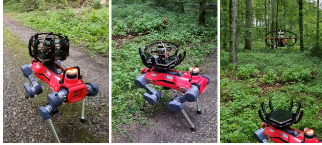
Fig. 10: Deployment of a marsupial mission, including (left to right) the walking phase on easy terrain, the carrier mechanism opening, and the aerial robot starting the exploration mission.
