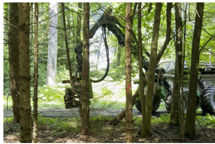
Fig. 19: The SAHA robot releases the cut tree after manual triggering.
