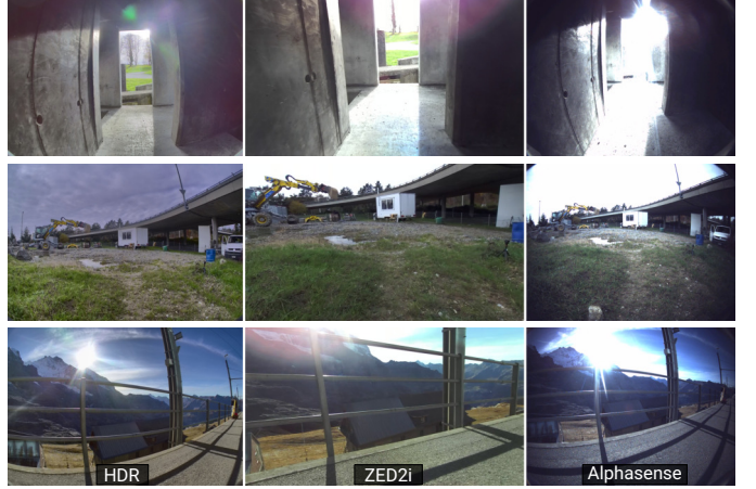
Fig. 10: Image Quality Comparison. The HDR camera excels in dark and low-light conditions. The ZED2i misses details in challenging scenarios (Row 1: Tree, Row 2: Sky). The CoreResearch struggles with overexposure and misses crucial details that are essential for localization.
