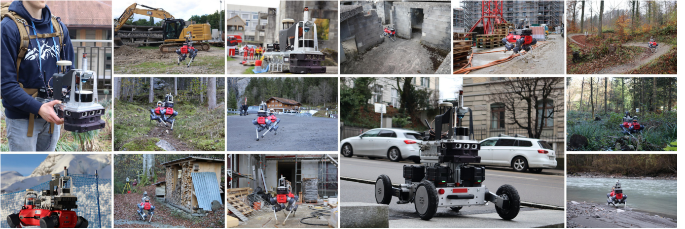
Fig. 1: Boxi can be deployed handheld, on a legged robot, or a wheeled robot across a variety of environments.
